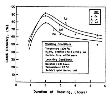
Fig. 4. Effect of the duration of roasting on the leach recoveries of rare earths
