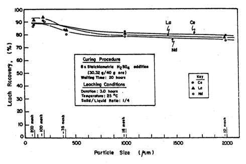
Fig. 2. Effect of the particle size of the sample on the leach recoveries of rare earths
